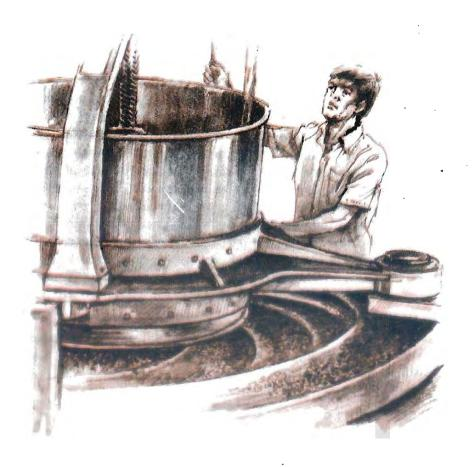
"As you can see in C.T.C. manufacture the leaves are completely shredded, and the juice squeezed out and evenly mixed. So the colour is brought out. In Orthodox, where there is no cutting, the juice is brought out slowly, so the flavour remains."
